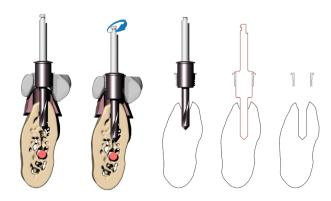
EXAMPLE OF USING THE DRILL Ø 2.3 x 11.5 mm 3DM613.23.115
